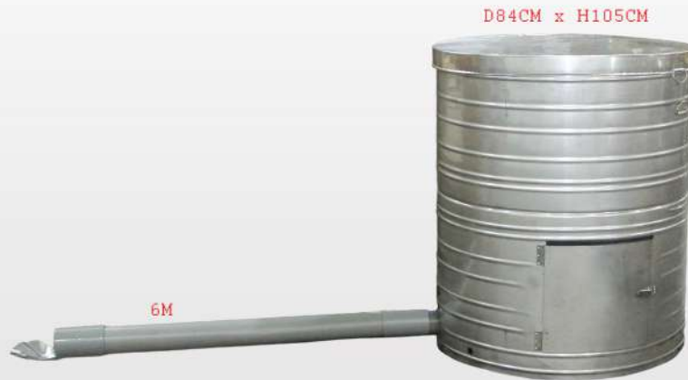
HA-320 (1/2HP, 1PHS, 220V, 50HZ, CAPACITY 180KG) (FOR BIGGER FEED PELLET UP TO 20MM)
